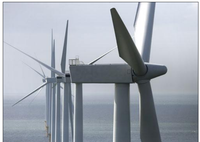
Fig. 1 Siemens SWT-3.6-107 wind turbine installed in an offshore wind farm (powergeneration.siemens.com).
