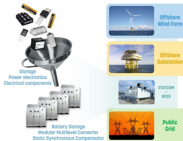
Figure 1 Simplified representation of a WPP setup with a BESS unit and MMC STATCOM onshore.
